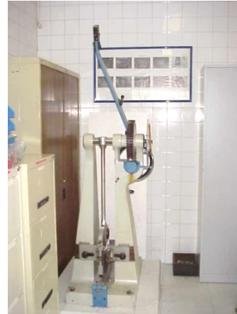
Charpy tests machine
