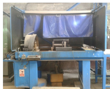
Magnetic test installation (TIEDE)
